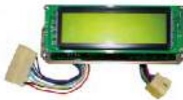
Battery Display Board
